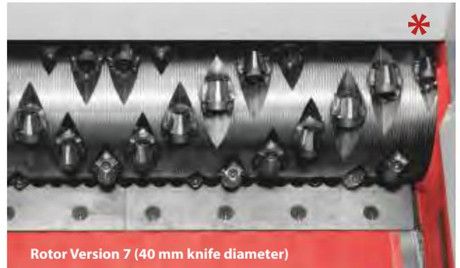
The highly efficient scissors cut of the concave ground circular cutting heads provide a very high work rate with very little effort. The knife holders are welded or mounted on the rotor and the round knives can be turned up to **8 times** with just a few adjustments before having to be exchanged completely. The use of various types of knives enables job-related adjustment of the shredder to the material being processed.
