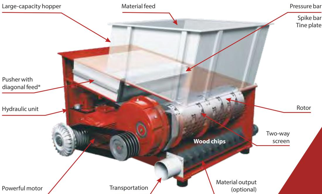
\* The wood chips fall into the rotor faster by force of gravity
